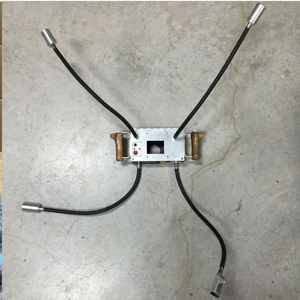
Photogrammetry tool with 4 flexible flashes
