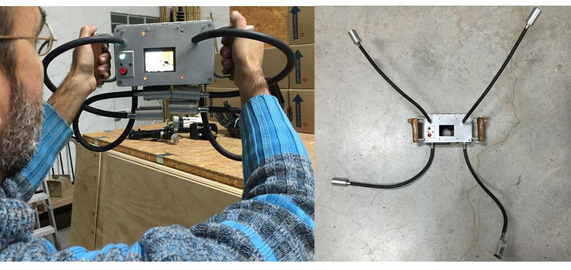
Photogrammetry tool with 4 flexible flashes size when folded : 55cm x 20 cm x 35cm
