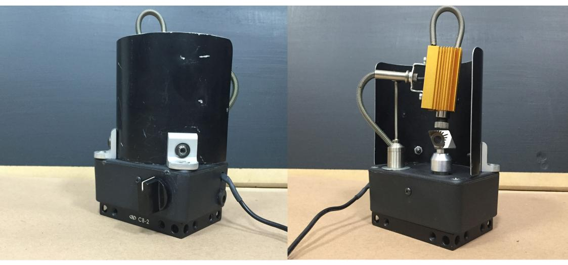
450µm 2W laser scanner with rotating mirror size: 15 cm x 10 cm x 25 cm
